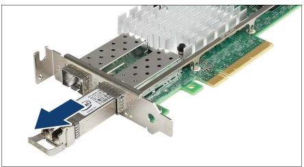
Figure 44: Removing the SFP+ transceiver
